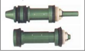
There types of contaminants can often be identified by their smell in the master cylinder reservoir or by corrosion. Flush the system, and then replace all rubber parts including caps, seals, and hoses.
