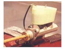
This reduces lost pedal travel but it means before the retaining nuts are tightened, there will be a small gap between the master cylinder and the booster. Once the cylinder is refitted, the bleeder pipes can be taken off and the brake lines re-connected.
