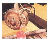
A tip. Always loop the bleeder hose up above the bleeder screw before it's immersed in the container of fluid. This makes it easier to see the air leaving the system and it always leaves a head of fluid at the bleeder screw, too.
