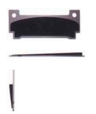
The pad on the piston side can wear concave. This is caused by the backing
