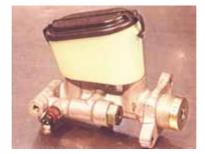
The brake lines will have a little air left in them so they shouldn't be fully tightened. Get rid of this air by having someone push slowly on the brake pedal until a steady stream of
