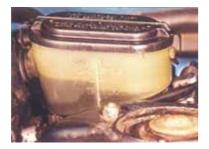
Often the cause is simply that the fluid is leaking from somewhere in the system. It's usually pretty easy to find the leak if there is one – and once found it should be fixed straight away. Once the leak has been fixed, refill the system with the correct grade of brake fluid, then bleed the system.
