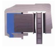
plate flexing under repeated heavy braking. If the dimple on the back of the rear disc pad is incorrectly positioned so that it does not line up with the slot in the piston, then the pad will flex when the brakes are applied, giving a spongy feeling to the brakes.
