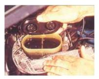
There are two different reasons for this depending upon the cause. In the case of air in the system, the air will have been compressed when the pedal was pushed down. When the pedal was released, the air will have expanded forcing the fluid up the brake lines more quickly than normal.
