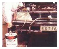
The brake system is then pressurised by a pump that is connected to a drum of new brake fluid. Each bleeder screw is opened and closed in turn until the system is free of air. The adaptor can then be taken off the master cylinder and
