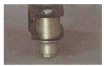
The load sensing proportioning valves are often used on vehicles which operate with widely differing rear axle loads, such as wagons and bakkies.
