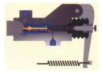
When the driver presses on the brake pedal, fluid enters the inlet port, travels through the hollow piston, past the poppet valve and out to the rear brakes.
