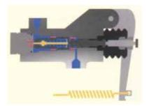
When the force developed by the fluid pressure action on the large area of the piston overcomes the combined forces of the small area the pressure spring, the piston moves to the left.
