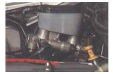
Along with these different mountings also comes different types of proportioning valves. Valves may be either single, or dual pressure sensitive, or pressure sensitive with a bypass feature, that allows full pressure to the rear brakes should the front hydraulic system fail.
