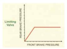
These valves, whilst an improvement, still prevented the rear brakes working at their optimum under all braking conditions.
