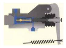
The small spring acting on the poppet valve now pushes it to the right, sealing the passage to the rear brakes.
