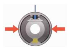
This in turn causes the wheel cylinder to move further than it normally would, requiring more fluid from the master cylinder and resulting in longer pedal travel.
