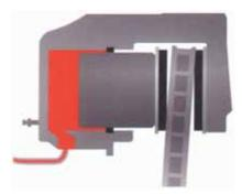
This naturally results in increased piston movement, making the master cylinder displace more fluid and leading to an increase in pedal travel.
