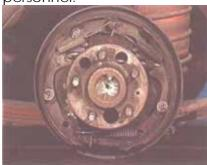
Should this be the case the only long term solution to the problem is to refit the self adjusting mechanisms.
