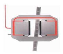
Again we are faced with increased travel to bring the pads into full contact with the disc and again the master cylinder must displace more fluid.
