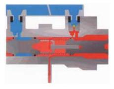
This extra displacement is controlled by the fast fill valve.
