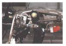
Whilst new vehicles should not suffer form this problem, older vehicles which have been in service for some time should have their pedal pivot points and linkages examined for excessive movement.
