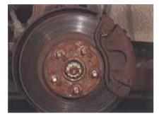
When brake drag is encoutered customer concerns usually centre around a lack of vehicle performance and an increase in fuel consumption.
