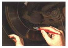
Our third and final check is to make sure that all wiring is held in it's correct position in the vehicle, and that none of the electrical plugs in the wiring loom, or into the modulator and ECU, have come loose.
