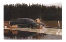
This usually causes the wheels to lock, resulting in a loss of vehicle stability and steearing control.
