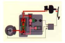
The ECU, as we have already stated constantly monitors wheel speed, but will not activate the modulator until it receives an input signal from one or more of the wheel sensors, telling it that a wheel, or wheels, are close to lock-up.
