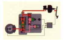
Should the ECU continue to receive signals from the wheel speed sensor telling it that the wheel is still slowing down at too fast a rate, it will then further increase current flow to the solenoid. This then moves the valve assembly the second half of it's stroke and connects the caliper to the accumulator circuit.
