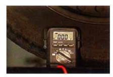
An assistant can now spin the wheel by hand, and if the sensor is functioning correctly a small AC voltage should be shown on the meter.
