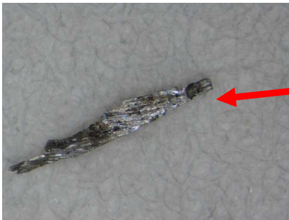
Aluminum swarf causing leakage from gear side
