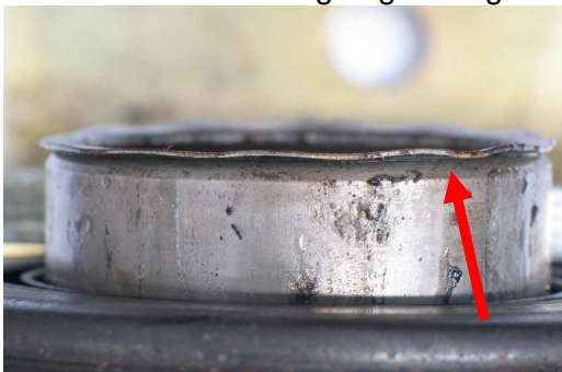
Over-stroke retaining ring damage
