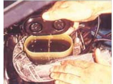
There are two different reasons for this depending upon the cause. In the case of air in the system, the air will have been compressed when the pedal was pushed down. When the pedal was released, the air will have expanded forcing the fluid up the brake lines more quickly than normal.
