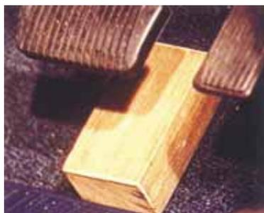
Remember that the problem of dirt in the piston bores still applies here. It pays to place a chock under the pedal to limit the distance it travels.
