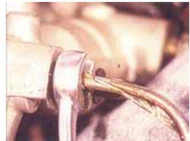
Once the cylinder is bled, take it out of the vice and refit it to the vehicle. Most Australian produced vehicles use the booster output rod as the stop for the master cylinder pistons.
