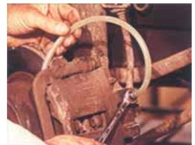
Tighten the bleeder screw and release the brake pedal to the rest position. Repeat this until only clean fluid with no air comes out the bleeder screw.
