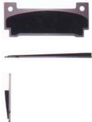
The pad on the piston side can wear concave. This is caused by the backing
