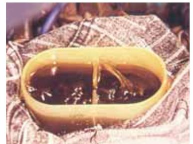
Alternatively, if the brake drums are oversize or the brake pads are incorrectly aligned, the abnormal deflection in the system will displace more fluid
