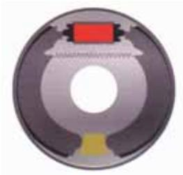
The special grinding of the shoes is called radius grinding, and it stops the shoes from contacting at the ends first, which would cause squealing and grabbing.
