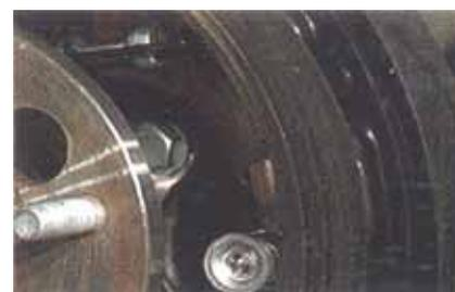
Disc brakes are likewise susceptible to oil or grease contamination, and should also be checked for the correct lining material being fitted. A significant increase in the co-efficient of friction of a lining
