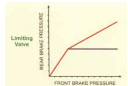
This would then allow the rear brakes to work at their optimum throughout the braking
