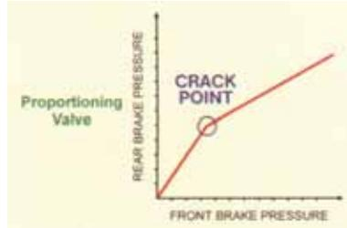
This crack point is controlled by the strength of the pressure spring, and there are different springs to suit different applications.
