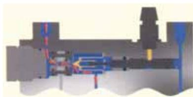
At this stage, the pressure delivered to the rear hydraulic cylinders is totally controlled by the driver pressing on the brake pedal.
