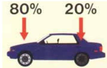
In the majority of cases up until the early seventies this ratio split was determined by the relative sizes of front and rear hydraulic cylinders, and brake design alone. To maintain vehicle stability brake engineers designed a system that would minimise rear wheel lock up under maximum braking force conditions.
