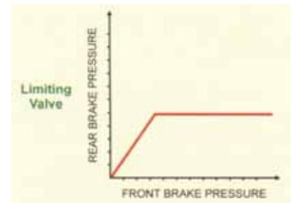
These valves, whilst an improvement, still prevented the rear brakes working at their optimum under all braking conditions.
