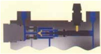
Early systems saw the valve inserted in the line to the rear brakes, and some modern front wheel drive vehicles still mount their proportioning valves remotely on the vehicles bulk-head.
