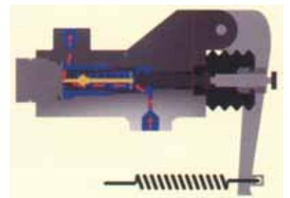
When the driver presses on the brake pedal, fluid enters the inlet port, travels through the hollow piston, past the poppet valve and out to the rear brakes.
