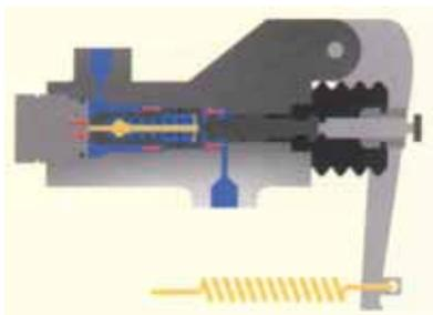
When the force developed by the fluid pressure action on the large area of the piston overcomes the combined forces of the small area the pressure spring, the piston moves to the left.
