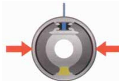
This in turn causes the wheel cylinder to move further than it normally would, requiring more fluid from the master cylinder and resulting in longer pedal travel.
