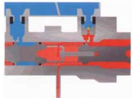
This extra displacement is controlled by the fast fill valve.
