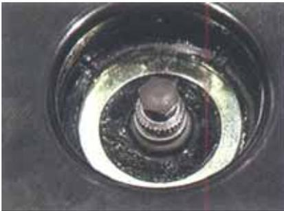
On non adjustable systems a component mismatch, or the use of non genuine replacement parts will most likely be the cause.
