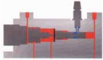
This will be easily detectable due to the increased eruption, or turbulence, visible in the reservoir as the pedal is first depressed.
