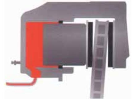
This naturally results in increased piston movement, making the master cylinder displace more fluid and leading to an increase in pedal travel.
