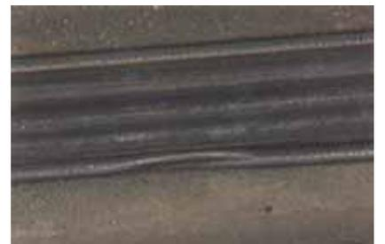
Flexible hoses can become damaged and twisted when calipers are replaced after being overhauled or having pads replaced.
