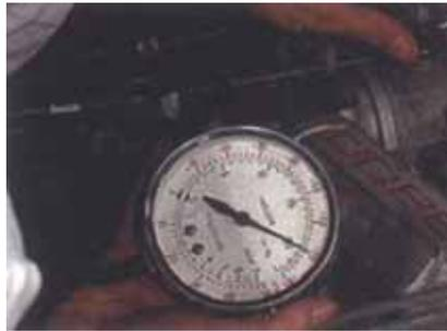
Low manifold vacuum could be an indication of internal problems in the engine, inlet manifold leaks, or an engine which has been highly modified with a non-standard camshaft.
