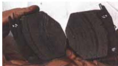
Burning is easily recognised as the linings will appear black and usually have deep cracks over the surface of the material.
