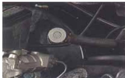
With the engine running remove the check valve from the booster, or in the case of vehicles with in-line check valves, the hose from the booster.
