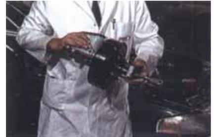
A common practice amongst some service personnel when faced with low pedal problems is to fit a master cylinder of a larger diameter than was originally fitted to the vehicle.
