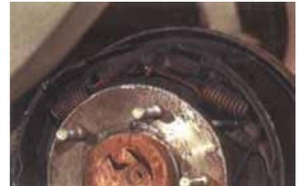
If the problem has only occurred since the brakes were re-lined the cause may be that the pads were not bedded in properly, or not bedded in at all.
