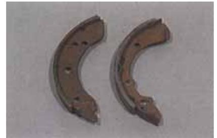
A brake shoe must have a certain amount of flexibility which will allow it to conform to the shape of the drum during braking. Making the shoe flex ensures even contact over the whole shoe and not only reduces noise but also increases braking force.
