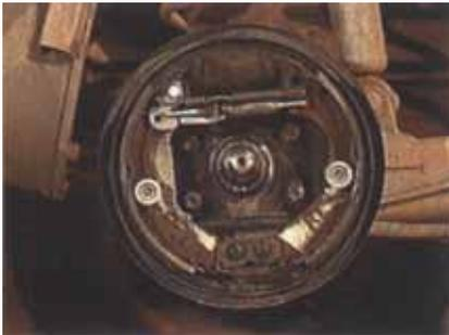
It's worth noting here that even with these clips and anchors to reduce shoe vibrations, most manufacturers recommend that some form of high viscosity lubricant, such as caliper slide grease, be applied to the shoe ends and where they contact the backing plate.
