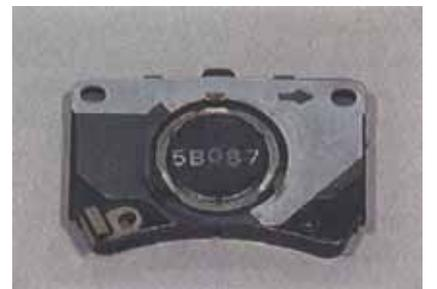
These shims are usually marked in some way to facilitate correct assembly and may also require the use of some form of lubricant in
