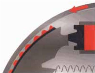
The final noise we shall look at is hum. Hum is usually associated with rear disc calipers and only occurs at low speeds, often when reversing.
