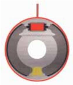
Applying the handbrake causes that portion of the drum where the shoes contact to cool at a different rate, leading to distortion and judder.
