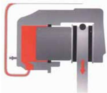
Modern disc brake pads have anti-squeal material bonded to their backing plates but may also employ an additional steel shim on the piston side pad.
