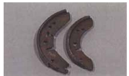
Also of significance in the reduction of noise is the way the shoes are located against the backing plate. Brake shoes are commonly
