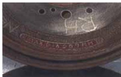
Drums need to be checked for size before and after machining. They should also be the same diameter on both wheels of an axle and if oversized replace in pairs.
