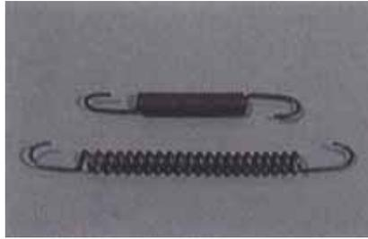
Should any of these be present, the springs or clips should be replaced in sets for both wheels on the axle.
