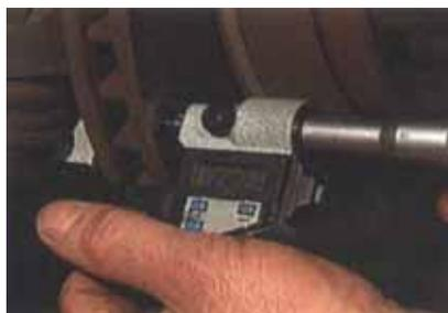
Rotors should be checked for run-out using a dial indicator and thickness variation, preferably using a micrometer for accuracy. In the absence of these, a
