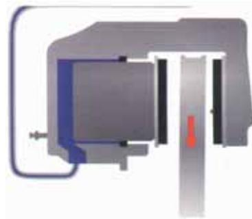
Rotor thickness variation can be generated by insufficient pad retraction or binding sliding calipers. This allows one pad to stay in contact with the rotor in the released position, causing the rotor to wear unevenly.
