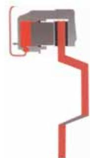
This uneven cooling causes the rotor to distort, which means it then has run-out and eventually judder.
