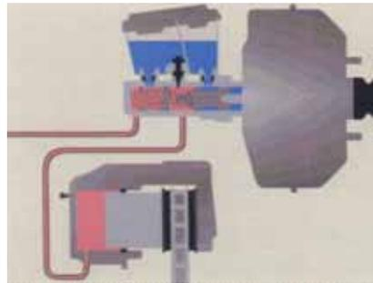
If the fluid now drips freely from the master cylinder port the adjustment of the pedal push rod and stop light switch will need to be checked and adjusted to manufacturers specifications as necessary.
