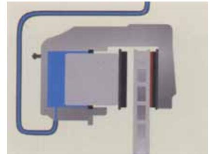
If this condition exists then the slides from both calipers on the axle should be removed, cleaned and lubricated.
