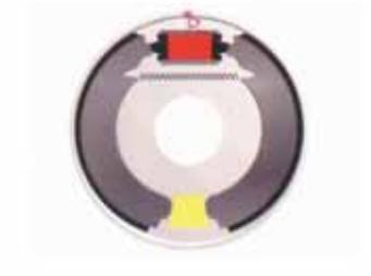
The most common type of rear drum brake assembly
