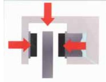
When the driver puts the brakes on, pressure from the master cylinder forces the pads against the rotor. The resulting friction develops the braking force needed to slow or stop the vehicle. The force with which the pads clamp the rotor governs the amount of brake force generated.
