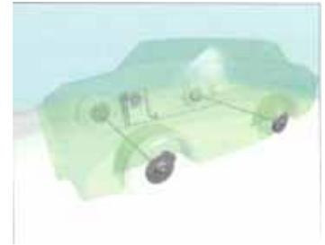
Whilst some master cylinder pistons are operated by a push-rod connected to the brake pedal, most have a power brake booster that helps the driver by increasing the force on the piston, and reduces the driver's pedal effort.
