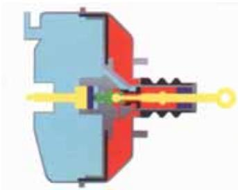
A control valve regulates the amount of atmospheric pressure let into the rear chamber. Operated by the pedal pushrod, the valve is directly connected to the output pushrod, and includes a vacuum valve.
