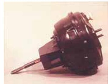
There is a vacuum in the manifold of all four stroke petrol motors. Brake boosters use this to increase the force applied to the master cylinder by three to five times without losing brake sensitivity or response. On diesel engines, an
