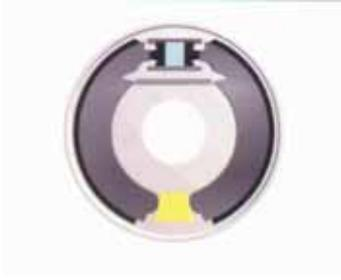
The pressure with which the shoes are forced against the drum controls the amount of friction heat and hence the braking force.
