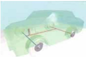
If there's a failure in one circuit, the amount of available braking force corresponds to the amount of weight on the axle. Front engine rear wheel drive vehicles usually have 60% of their
