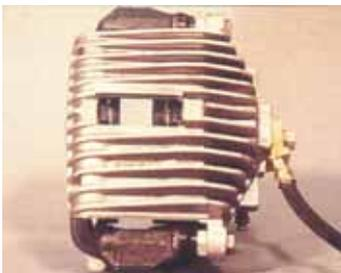
While fixed head calipers may have four opposed pistons, some floating head calipers have two. Multiple pistons are used when more force is needed, like heavy or
