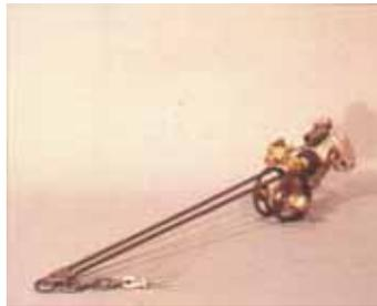
When a vehicle brakes, its weight is transferred to the front. The nose will dip as it gets heavier, and the rear will raise as it gets lighter. The rear wheels need less hydraulic pressure, hence the purpose of proportioning valves.
