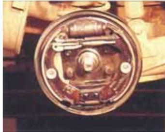
Both types provide a parking brake operated by a driver's lever connected via cables to a lever-and-strut mechanism that expands the brake shoes against the drum.
