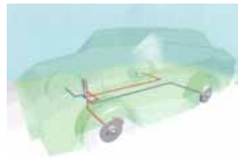
This has one front wheel and the diagonally opposite rear wheel connected to each circuit. Should either circuit fail, an equal amount of braking will still be available.
