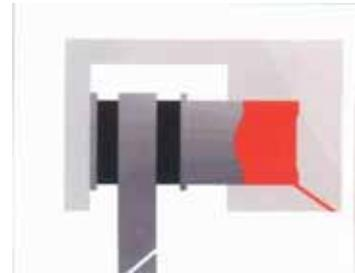
Most of the rotor is exposed to the air so friction heat is easily radiated away. This minimises brake fade and helps keep the braking stable at all speeds.
