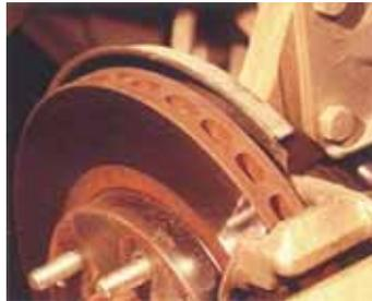
Disc brakes don't need periodic brake adjustments (to keep the distance between the pad and the rotor constant) because they adjust automatically in use.
