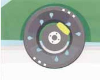
The disc caliper holds one or more pistons which force the pads against the disc rotor. Calipers may be either :
