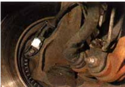
As we previously mentioned, the wheel speed sensors produce an AC voltage signal of varying magnitude and frequency which can be easily checked using a digital multimeter.
