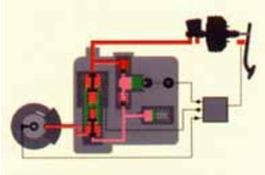
Should the ECU continue to receive signals from the wheel speed sensor telling it that the wheel is still slowing down at too fast a rate, it will then further increase current flow to the solenoid. This then moves the valve assembly the second half of it's stroke and connects the caliper to the accumulator circuit.
