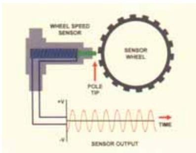
These AC signals are then sent via electrical cables, to the ABS electronic control unit, which uses them to calculate vehicle and wheel speeds.
