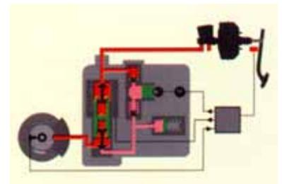
The ECU, as we have already stated constantly monitors wheel speed, but will not activate the modulator until it receives an input signal from one or more of the wheel sensors, telling it that a wheel, or wheels, are close to lock-up.
