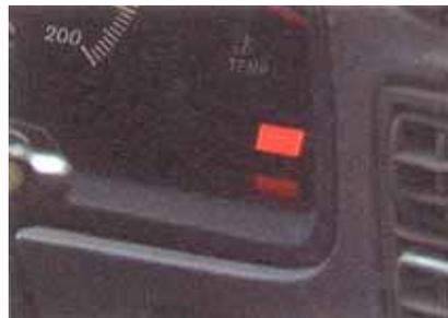
Behind all this is a sophisticated software program in the ECU which, when the vehicle first moves off after being started, runs the pump, cycles the solenoid valves and checks the signal coming from the wheel speed sensors, illuminating the warning light should a fault be detected. After this the ECU constantly checks the system, and should any faults appear, immediately switches the
