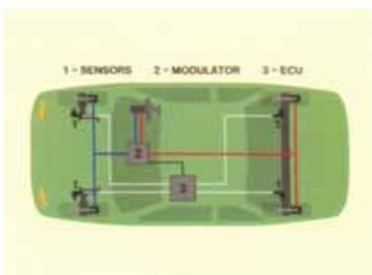
Front wheel drive, high performance and luxury vehicles, including four wheel drive vehicles, may have four channel, four sensor systems fitted. As the name implies, these systems control all four wheels individually, and may include additional sensing devices to further adjust hydraulic pressure to compensate for high lateral loads during cornering.
