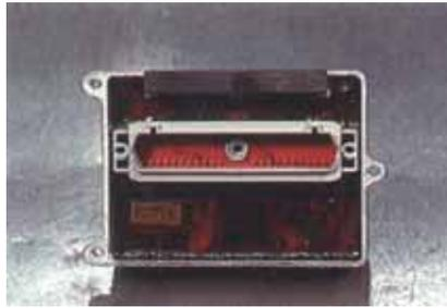
The ABS electronic control unit, which constantly processes signals from the wheel speed sensors, calculate the optimum wheel slip for maximum braking, and then control the hydraulic pressure delivered to the brakes by operating the solenoid valve housed in the modulator assembly.
