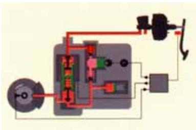
At this time the pump motor is also turned on by the ECU and brake fluid released from the caliper is returned to the master cylinder, causing the brake pedal to "kick back".
